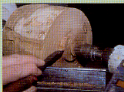
2 Turn the tailstock end flat and prepare it for your faceplate or four-jaw chuck
