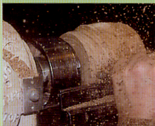
3 With the bowl mounted in a chuck, use a bowl gouge to start shaping the bowl
