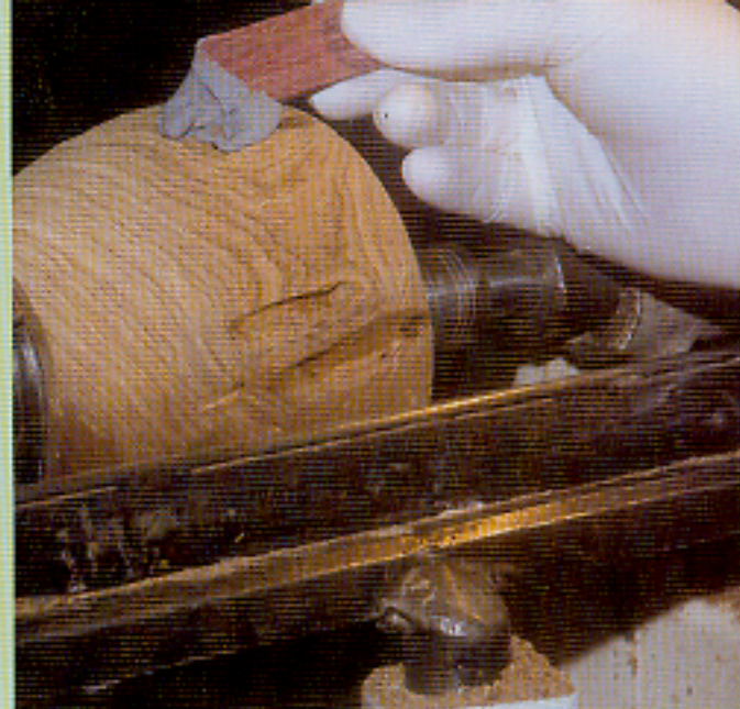
7 Using a spatula, force the filler material into the flaws
